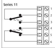
Series 11 denotes a ReSet call point that incorporates two independent single pole changeover switches providing double pole changeover contacts. Easily accessed through the installer terminals as illustrated.
