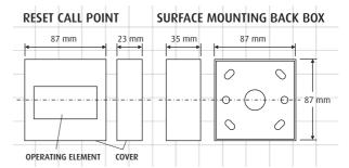
ReSet components and technical information **FLUSH MOUNTED** SURFACE MOUNTED RESET CALL POINT SURFACE MOUNTING BACKBOX - COLOUR MATCHED (OPTIONAL) WALL PLATE WALL PLATE OPERATING ELEMENT COVER SCREW 3.5 x 35 OPERATING (2) PROVIDED RESET KEY
